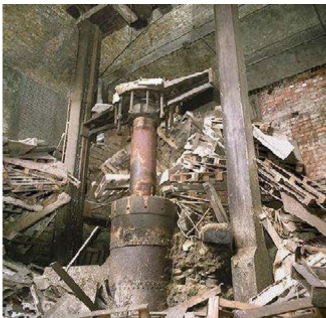
Fig 6.3.29: The hydraulic accumulator [clockwise from top: view from London Road; surviving columns; historic image with debris]
